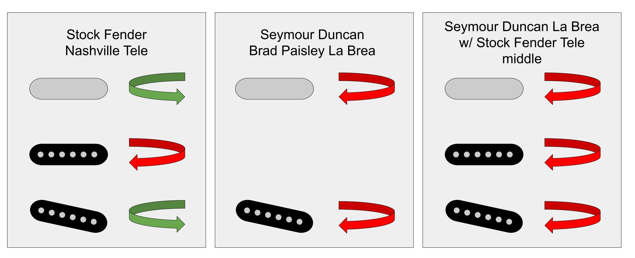
Seymour Duncan pickups are wound in the opposite direction as the Fender Nashville neck and bridge pickups. Replacing a standard Tele pickup set with these is fine because everything is reversed.
